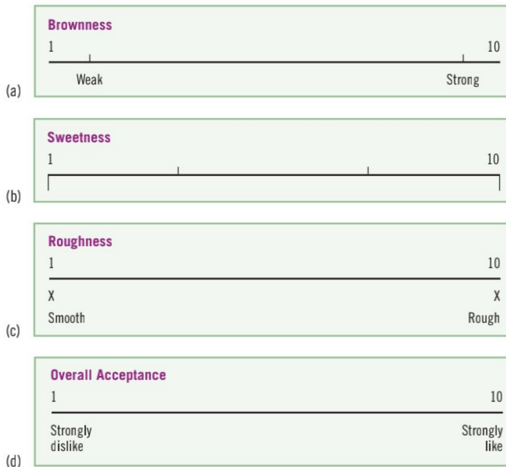
FIGURE 3.4 Examples of line scales. (a) Brownness. (b) Sweetness. (c) Roughness. (d) Overall acceptance.
